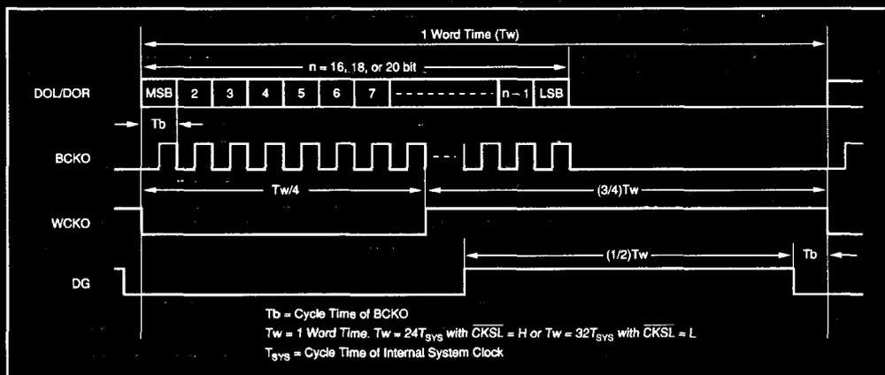
FIGURE 3. Output Data Timing Waveforms.
